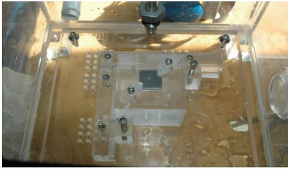
**Figure 1. Nozzle and sample holder in DYNFLOW’s “7 ksi - 5 gpm” cavitation jet erosion test loop.**
