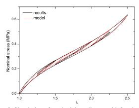
Figure 2: Simulation of a uniaxial tensile test with four hysteresis loops (nc1 test).
