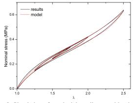
Figure 3: Simulation of a uniaxial tensile test with a hysteresis loop inside another one (nc2 test).
