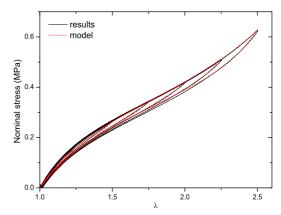
Figure 1: Simulation of a uniaxial tensile test with increasing cycle.
