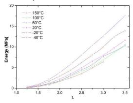
Figure 5. Energy corresponding to the hysteresis during the second cycle for the filled silicone at different temperatures.
