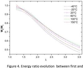
second loads versus the maximum elongation for different temperatures.
