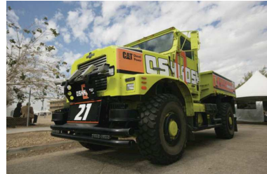
Fig. 1. TerraMax autonomous vehicle participant of the DARPA Urban Challenge which used a stereo vision system to urban environment perception [3].
