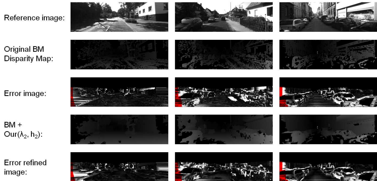
Fig. 6. Result for the Disparity map refinement of the BM method in different urban conditions.
