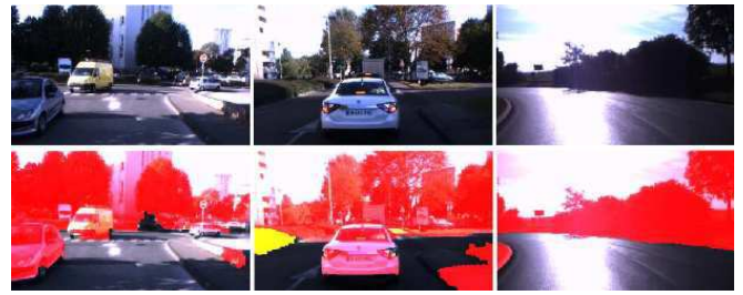
Fig. 9. The original image on top and the classification results on bottom for extreme conditions, where original colour represents the road detected, the red pixels are the non-road surfaces, and the yellow ones representing the unknown areas.
