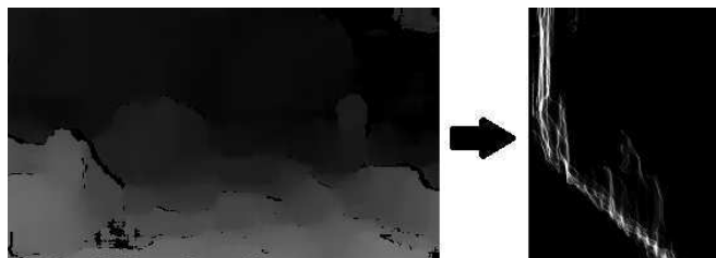
Fig. 4. The disparity map from the stereo pair of Figure 2 (left), and the v-disparity map (right).
