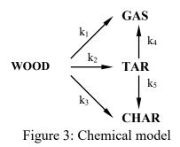
The wood is decomposed by three simultaneous primary reactions producing a solid carbonaceous residue (the char), a pseudo species of condensable gases (the tar) and a pseudo species of noncondensable gases (the gas). The secondary decomposition of the tar produces more gas and char. The reaction constants obey the Arrhenius formalism and the kinetic data is presented in Table 1.
