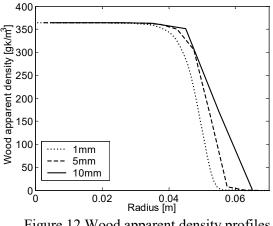
Figure 12 Wood apparent density profiles (t=1200s, dt=0.1s) (300x70 nodes)
