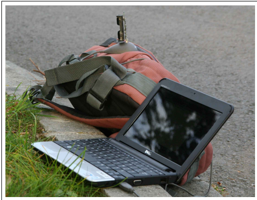
Fig. 5 One base station (i.e. netbook + TELOS-B mote) installed on the roadside during the running race at Ker Lann campus
