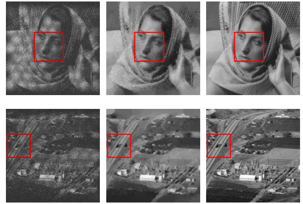
Fig. 4: Reconstruction of the images "barbara" (top row) and "factory" (bottom row) with a noise level \sigma = 0.1 . The remaining parameters are set as \bar{w} = 16.2 , \sigma_c = 0.81 and \sigma_w = 0.07 . The left column correspond to the available data where each pixel is assigned its maximum intensity over all laser shots. The middle and right columns correspond resp. to the image estimate and the ideal image.
