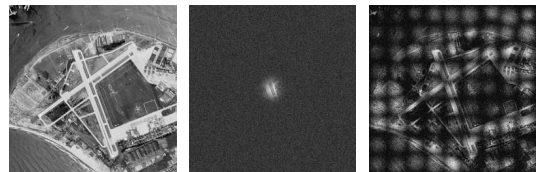
Fig. 1: Acquisition process in mosaic laser imaging. From left to right: the ideal image we want to estimate, a reduced part of the field of view with a single laser flash (laser shot), the image composed from all laser shots where each pixel is assigned with its maximum intensity over all of them.
