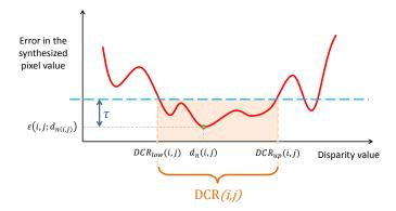
Figure 9: Definition of DCR for a given threshold  $\tau$ .
