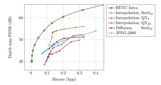
Figure 6: Rate-Distortion performance of the  $V_3$  first "breakdancers" depth map with different quality factors of JPEG-2000 and HEVC and different Sobel detection thresholds  $\lambda$  for the three proposed methods. The proposed methods differ in the interpolation from decoded edges and seeds: diffusion or bi-linear interpolation from regular seeds and bi-linear interpolation from quadtree-placed seeds.
