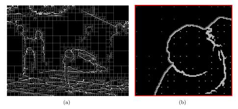
Figure 4: Ilustration of the quadtree decomposition on the criterion of edge presence.
