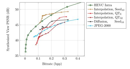
Figure 7: Rate-Distortion performance of synthesized  $V_4$  with the bitrate of  $V_3$  depth map, for different quality factors of JPEG2000 and HEVC, and different Sobel detection thresholds  $\lambda$  for the three proposed methods.
