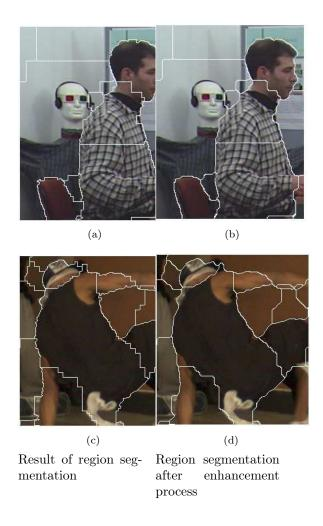
Figure 34: Region segmentation after applying enhancement process
