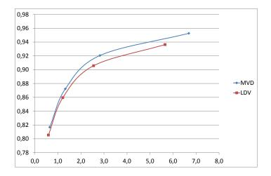
Figure 27: SSIM curves of the synthesis of viewpoint 3 of the *BDancer* sequence after compression of both MVD and LDV. Viewpoint 3 is an intermediate position which is synthesized for both representations.
