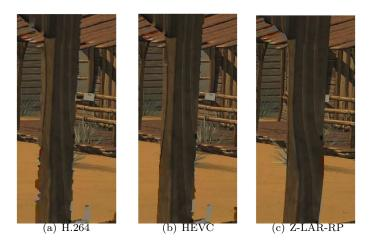
Figure 39: Snapshot of synthesized frame - GT\_Fly, 0.01bpp.
