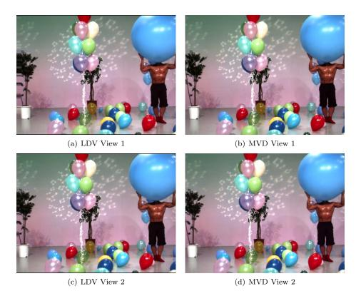
Figure 28: Balloons Sequence encoded at QP=25. Synthesis of viewpoint 2 with both representations. Viewpoint 1 corresponds to a decoded view in the MVD case whereas it is synthesized from the decoded LDV.
