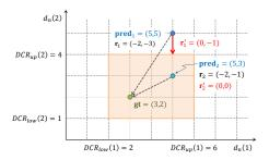
Figure 10: Coding the residuals using DCR with a toy example with just two pixels  $(d_n(1) \text{ and } d_n(2))$ . In conventional coding, given predictor (**pred**), one aims to reconstruct the original ground truth (**gt**). However, considering DCR, it is sufficient to encode a generally smaller residual, i.e. one that enables to reconstruct a value inside or on the border of the DCR (shaded area in the picture).
