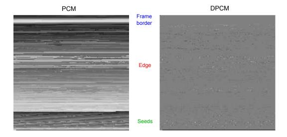
Figure 3: Illustration of the payload of the encoded pixels intensity values ("break-dancers" depth map). The PCM (left) pixel intensity and the DPCM (right) residuals are displayed in raster scan order.
