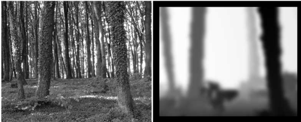
Figure 7: Original picture (a) and its disparity map (black areas stand for the closest areas whereas the bright areas indicate the farthest ones).
