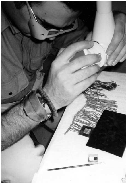
Fig. 1. Laser cleaning of fringes with silk core and tarnished gilt silver threads.
