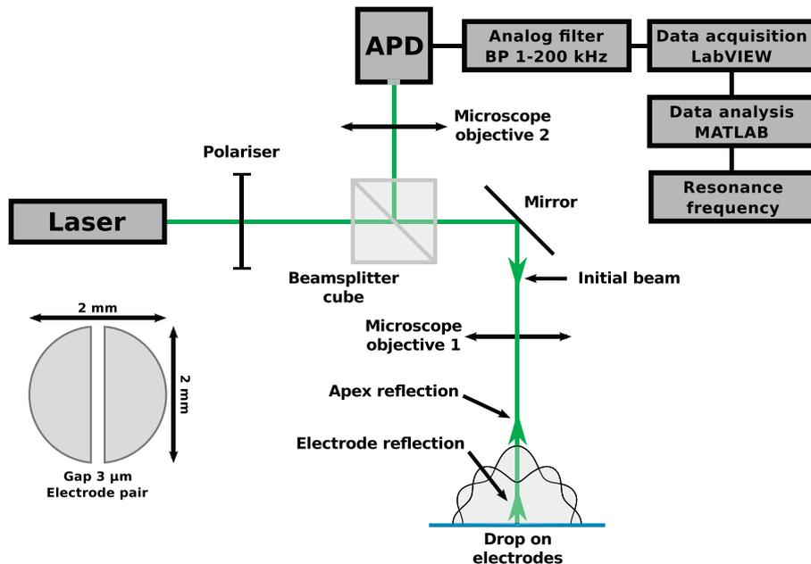
**Fig. 1.** Setup of the interferometry system. The laser beam crosses the optical system to form two reflections on the drop apex and the electrode, which are detected by the avalanche photo diode (APD). Insert: Electrode pair in use for electrowetting actuation.
