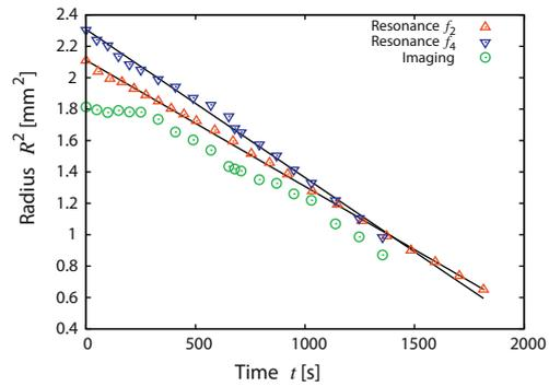
(b) The radius data is obtained via interferometry for mode 2 ( $\Delta$ ) and mode 4 ( $\nabla$ ), compared to imaging ( $\circ$ ). The measured evaporation times are  $\tau_{\text{evap},2} = 2627$  s and  $\tau_{\text{evap},4} = 2445$  s for mode 2 and 4, respectively.
