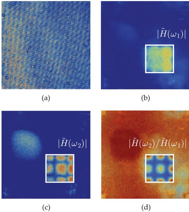
FIG. 3: Raw interferogram (a), hologram of statically-scattered light (central band), beating and  $\omega_1$  (b), hologram of the first modulation sideband beating at  $\omega_2$  (c), side-to-central band ratio (d). Colorbar in arbitrary logarithmic units.
