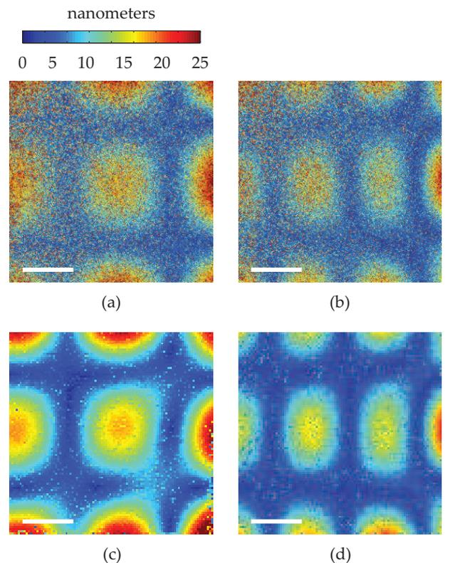
FIG. 4: Amplitude maps of the out-of-plane vibration of a thin metal plate versus excitation frequency  $\omega/(2\pi)$ . Holographic images at 40.1 kHz (a), 61.7 kHz (b). Scanning laser Doppler images at 40.1 kHz (c), 61.7 kHz (d). Scalebar: 5 mm.
