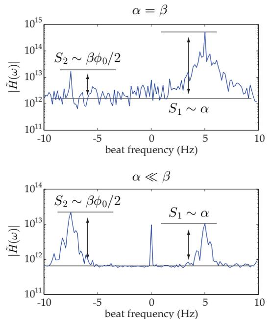
FIG. 2: Magnitude of the holograms  $\tilde{H}(\omega)$  (a.u., vertical axis) versus beating frequency  $\omega/(2\pi)$  (Hz, horizontal axis), averaged over the image of the piezo-electric actuator, for a vibration amplitude  $z_0 \sim 30$  nm. The top spectrum was acquired with a LO for which  $\beta = \alpha$ . For the bottom spectrum  $\beta/\alpha = 50$ .
