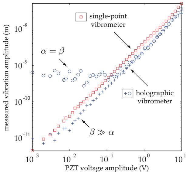
FIG. 5: Comparison of quantitative out-of-plane vibration amplitudes retrieved with the single-point laser vibrometer ( $\square$  symbols) and holographic vibrometer with  $\beta = \alpha$  ( $\circ$  symbols) and  $\beta \simeq 50\alpha$  ( $+$  symbols).
