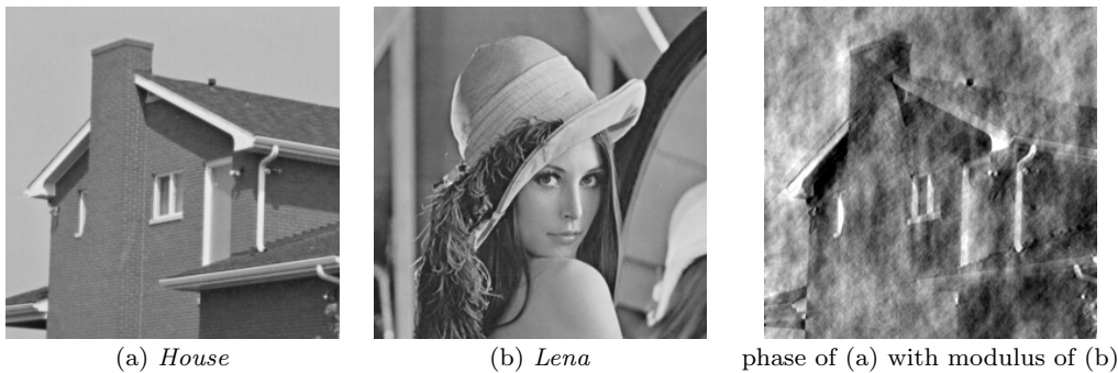
Fig. 1 Phase and perceived geometric content. When an image is built (in Fourier domain) with the phase of an image (a) and the modulus of an image (b), the perceived geometry is that of (a). This famous experiment of Oppenheim and Lim [30] shows that the geometry of an image is mostly encoded in the phase component.
