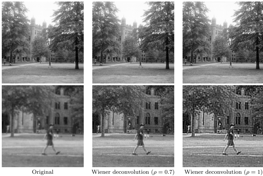
Fig. 9 Parametric blind deconvolution using sharpness indices. On the first row, we can see the original Yale image (left), and two Wiener- H^1 deconvolution results obtained with a kernel width of \rho = 0.7 (middle) and \rho = 1 (right). Close-ups of these three images are shown on the second row. The value \rho = 0.7 , which maximizes the sharpness indices SI and S (see Fig. 8), corresponds surprisingly well to the desired critical value that rules the transition between blur and ringing.
