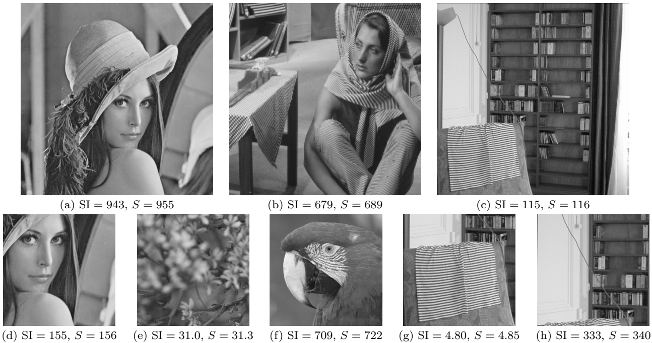
Fig. 5 Examples of values of SI and S for some natural images. One can observe that the values of SI and S are very close, and tend to be small for out-of-focus images like (e) and in the case of a strong high-frequency spectral component (g). Also, the order of magnitude of SI and S grows with the image size (compare the values for the 512 \times 512 images of the first row to those of the 256 \times 256 images of the second row), but it may happen that a sub-part of an image has a larger value of S (or SI) than the whole image, as in (c) and (h).
