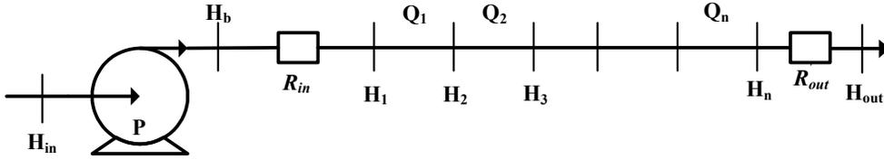
Figure 1: Schema of system Pump-Restriction-Pipeline-Restriction, the pipeline is dicretized in n sections.
