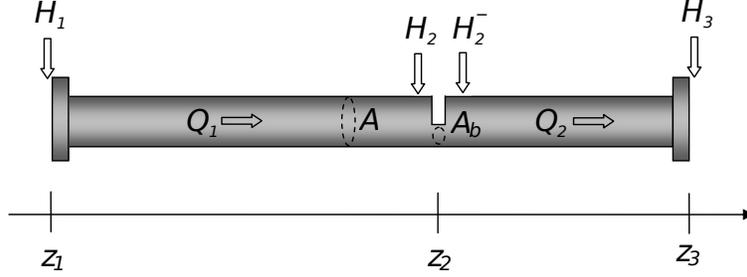
Figure 2: Pipeline discretized in 2 sections with a blockage at position  $z_2$  (begin of the second section).
