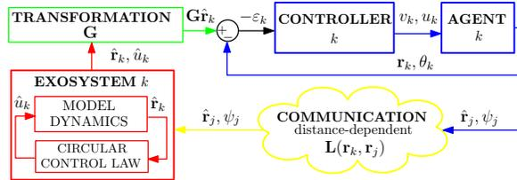
Fig. 1. Structure for the feedback design including a decentralized exosystem. Each agent  $k$  computes its own exosystem which communicates with other exosystems by means of a communication protocol depending on the distance between the agents (the Laplacian matrix  $\mathbf{L}$  depends on the agents' states  $\mathbf{r}_k$ ).
