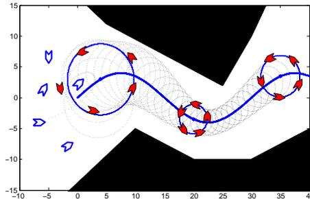
Fig. 3. Simulation of five agents governed by control law (15) with  $\mathbf{G}(t) = \mathbf{T}_{c(t)}\mathbf{S}_{R(t)}$ . The figure shows four snapshots: the initial conditions (blue void agents), a transient state at  $t = 40s$  and the stable uniformly distributed circular formation at  $t = 200s$  and  $t = 350s$ .
