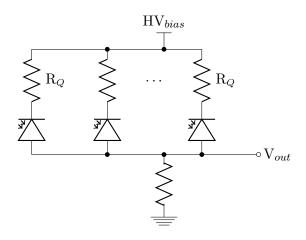
Figure 1. Electrical scheme of a SiPM showing the individual GM-APD and the quenching resistors  $R_Q$ . A small resistor (typically 50  $\Omega$ ) in series with the SiPM and the high voltage bias ( $\approx 70~V$  in the case of the MPPC) converts the current to voltage.
