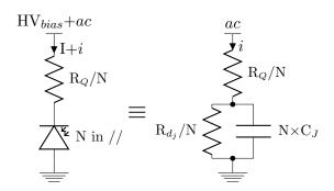
**Figure 8.** Small signal electrical schematic of a SiPM for ac measurement.  $R_{d_j}$  corresponds to the differential resistance of the GM-APD junction (without  $R_Q$ ).  $C_J$  is the junction capacitor.
