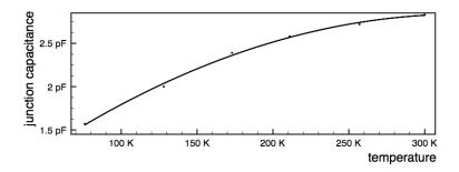
**Figure 10.** Junction capacitance as a function of the temperature. The measurement has been made with a 60 V biasing.
