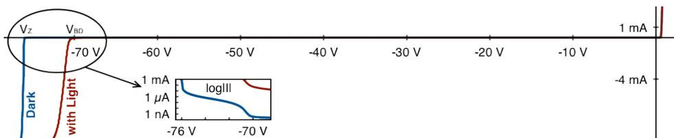
**Figure 3.** Typical SiPM  $I(V)$  characteristic at 300 K with and without incident photons. A zoom around the breakdown voltage is also shown using a log scale of the current absolute value.
