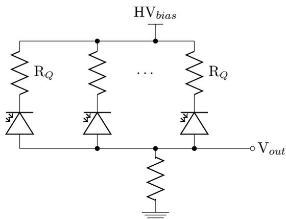
**Figure 1.** Electrical scheme of a SiPM showing the individual GM-APD and the quenching resistors  $R_Q$ . A small resistor (typically  $50 \Omega$ ) in series with the SiPM and the high voltage bias ( $\approx 70 \text{ V}$  in the case of the MPPC) converts the current to voltage.
