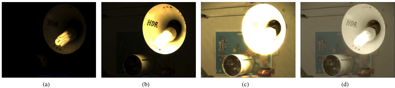
Fig. 6. Result of the complete system. Our Multiple Exposure Control can select the three proper exposures, and the specific memory management core permits us to display 3 bracketed images at the same time.
