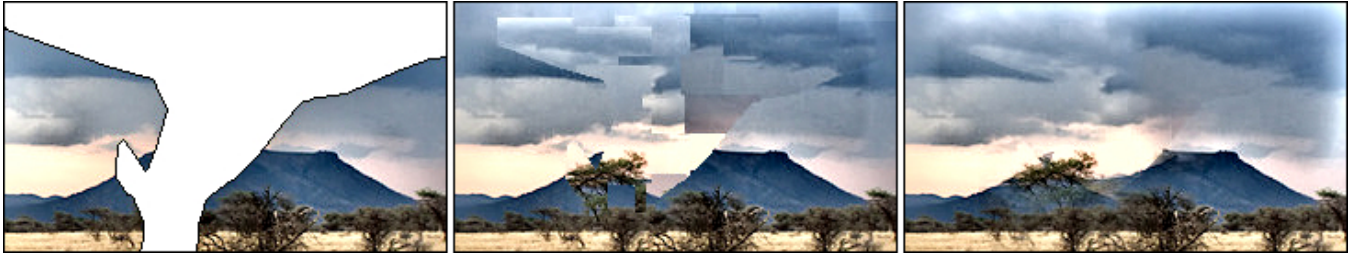
Figure 1: Illustration of our proposed spatial patch blending algorithm for image inpainting. From left to right : color image with area to reconstruct, reconstruction result with the inpainting algorithm from [Criminisi et al. 2004], our reconstruction result.
