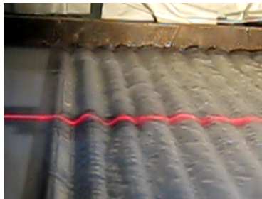
(a) Close-up photography of the experimental setup. The red line is the measured profile.
