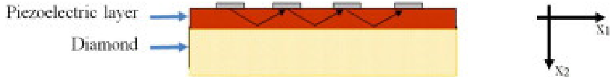
Fig. 1. Typical waveguide configuration considered for the dispersion analysis. The piezoelectric layer thickness is varied to find the best operating point.
