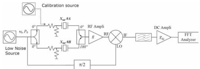
Fig. 1. Principle of the passive measurement bench.
