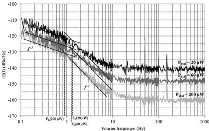
Fig. 2. The  $\mathcal{L}(f)$  of 5-MHz SC-cut resonators according to the dissipated power in the crystal. For  $P_{Xtal} = 20 \mu W$ , the cut-off frequency  $F_L$  is 1.4 Hz. For  $P_{Xtal} = 200 \mu W$ ,  $F_L$  is 0.8 Hz.
