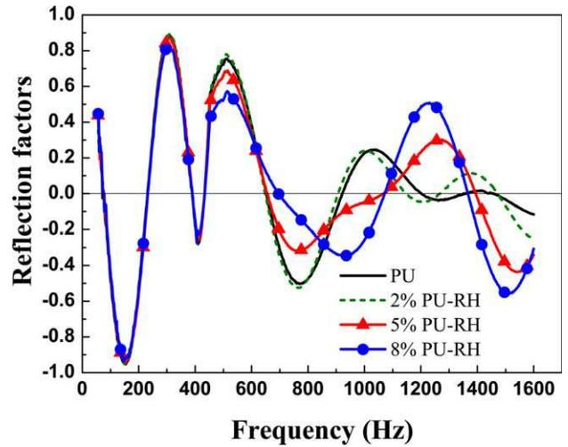
FIG. 8. The reflection factor of various foams. [Color figure can be viewed in the online issue, which is available at [wileyonlinelibrary.com](http://wileyonlinelibrary.com).]
