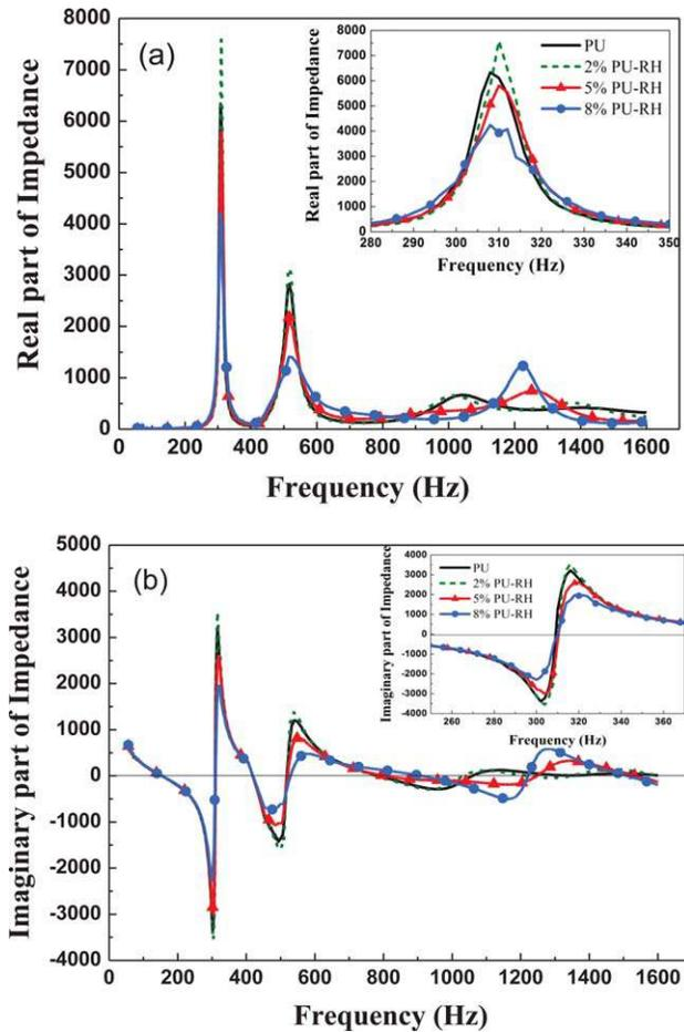
FIG. 7. The real part (a) and the imaginary part (b) of impedance for various foams. [Color figure can be viewed in the online issue, which is available at [wileyonlinelibrary.com](http://wileyonlinelibrary.com).]
