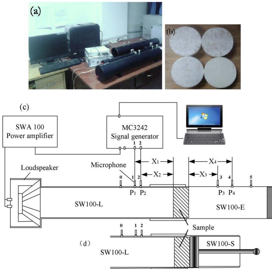
FIG. 2. The sketch map of test system of impedance tube. [Color figure can be viewed in the online issue, which is available at [wileyonlinelibrary.com](http://wileyonlinelibrary.com).]
