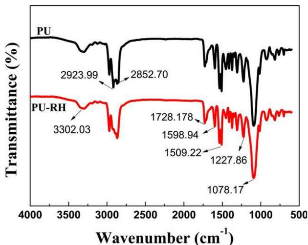
FIG. 3. ATR-FTIR spectra of PU and PU-RH composites. [Color figure can be viewed in the online issue, which is available at [wileyonlinelibrary.com](http://wileyonlinelibrary.com).]
