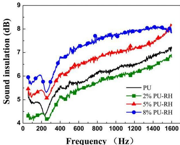
FIG. 10. The sound transmission losses of various foams. [Color figure can be viewed in the online issue, which is available at [wileyonlinelibrary.com](http://wileyonlinelibrary.com).]
