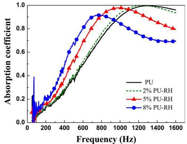
FIG. 9. The sound absorption coefficient of various foams. [Color figure can be viewed in the online issue, which is available at [wileyonlinelibrary.com](http://wileyonlinelibrary.com).]
