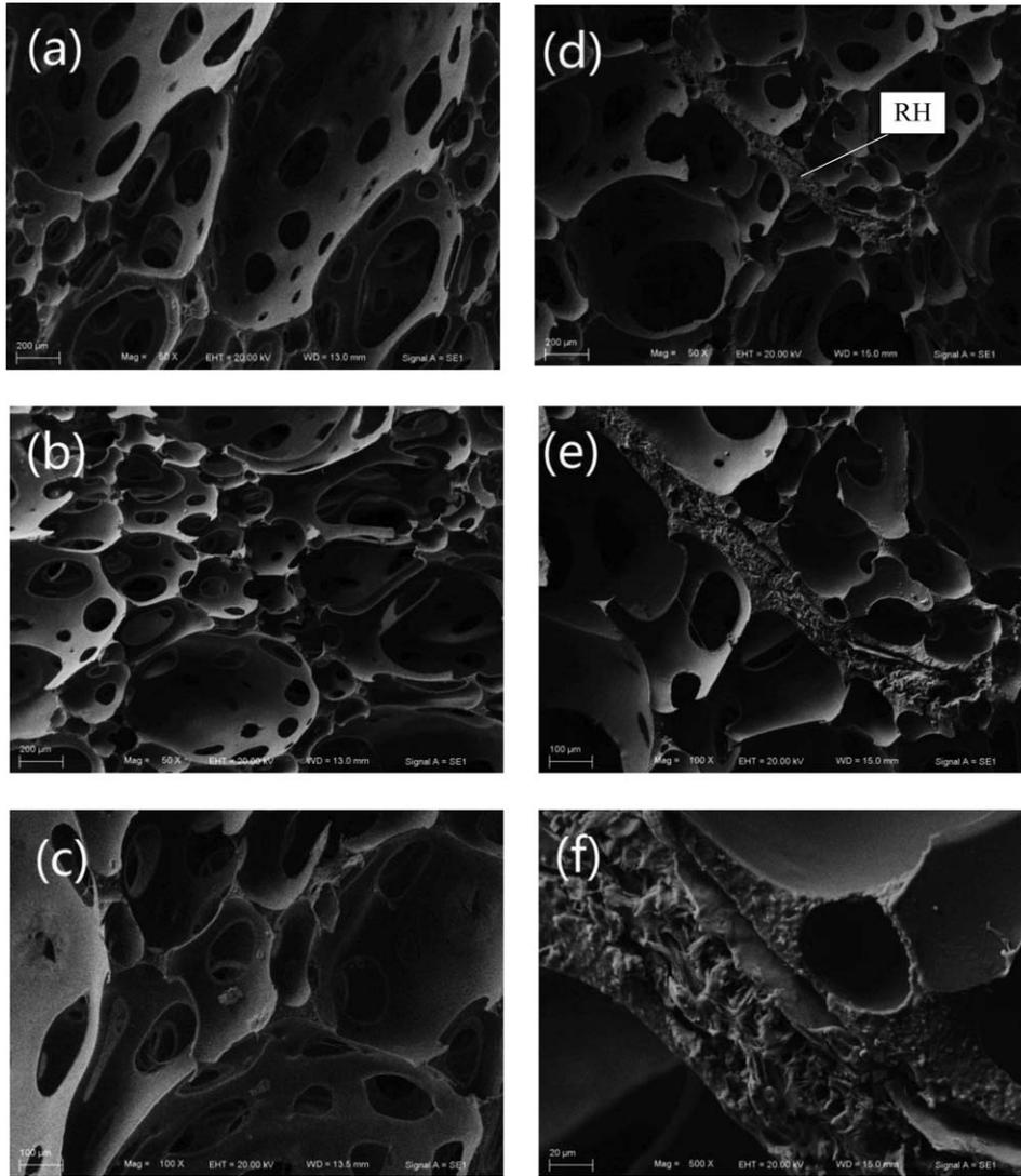
FIG. 5. Some SEM micrographs of PU-RH composites.
