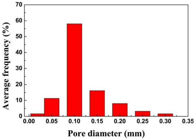
FIG. 6. Pore diameter distribution of PU foam. [Color figure can be viewed in the online issue, which is available at [wileyonlinelibrary.com](http://wileyonlinelibrary.com).]
