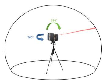
**Fig. 1** Operating principle of a terrestrial LiDAR (light detection and ranging) scanner (FARO Photon 120). A laser beam deflected by a rotating mirror scans a vertical plane, and the complete rotation of the device allows hemispherical scanning. This results in the digitisation and the representation of surrounding objects in a three-dimensional (3D) point cloud
