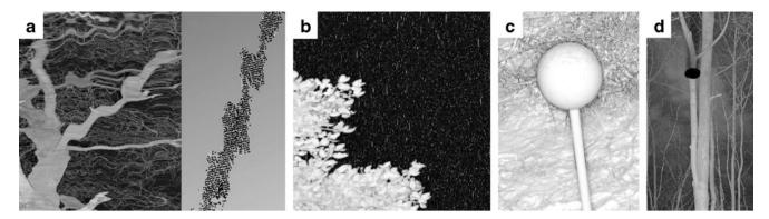
Fig. 4 Impact of climatic and sky conditions on scan quality. Wind leads to poor descriptions of tree axes (a), whereas snow intercepts laser beams and leads to an increase of noise points (b) and poor
