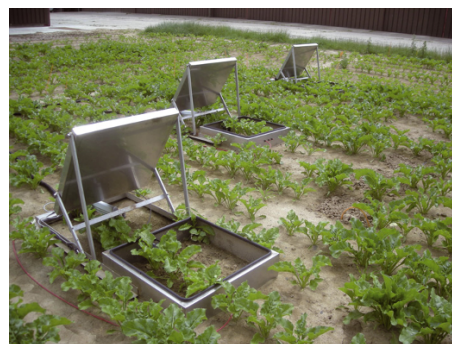
Measurement of N_2O and CO_2 fluxes with automatic chambers in a sugar beet plot, Estreets-Mons, June 2008 bessou©INRA
