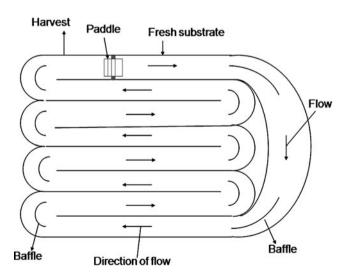
Fig. 2 Arial view of a raceway pond
