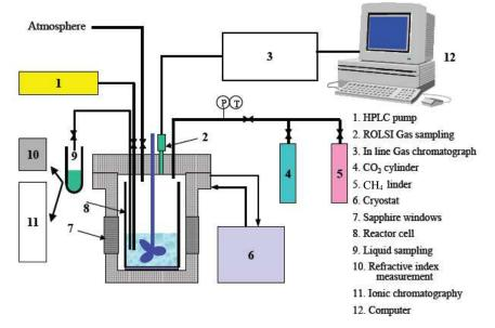
Figure2: Experimental device
