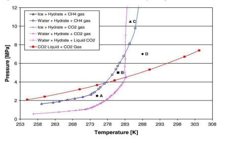
Figure 1. Equilibrium conditions of hydrate CO<sub>2</sub> and CH<sub>4</sub> (Naval Goel 2006)
