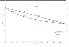
Figure 5 Phase diagram of hydrate CO2 - CH4 mixture at 2.2°C [ref sfgp:2013120099]-5
