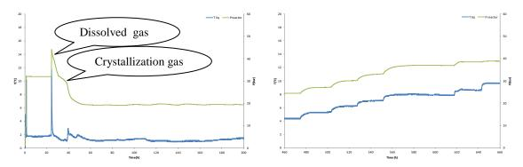
Figure 3 Evolution of pressure and temperature during crystallization and dissociation
