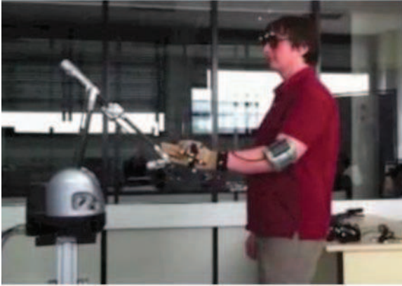
Fig. 8. Sensorimotor interfaces: haptic arm on the left, head and hand ART markers, cyberglove.
