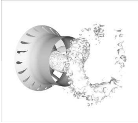
Fig. 11. Precessing vortex core (PVC) in cold flow LES visualized as a low pressure iso-surface.
