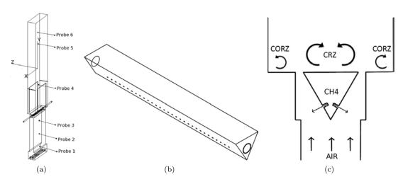
Figure 2. (a) Full burner geometry and location of pressure probes. (b) Wedge and fuel injection holes. (c). Cut of the burner around the fuel injection and flame stabilization zones.
