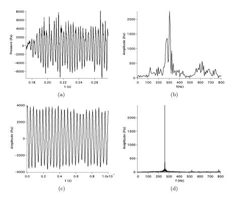
Figure 7. Pressure signals at probe 4 (Fig. 2(a)). Left (a) and (c): time signals. Right: (b) and (d): FFT. Top: LES (simulation 1), Bottom: Twente experiment. The LES data contains the initial growth phase from 0.18 to 0.22 ms. The experimental data corresponds only to the limit cycle variations.
