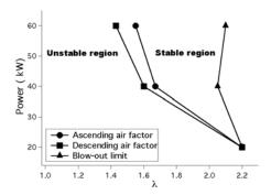
Figure 3. Stability map obtained experimentally showing the stable and unstable operation regions of the burner.
