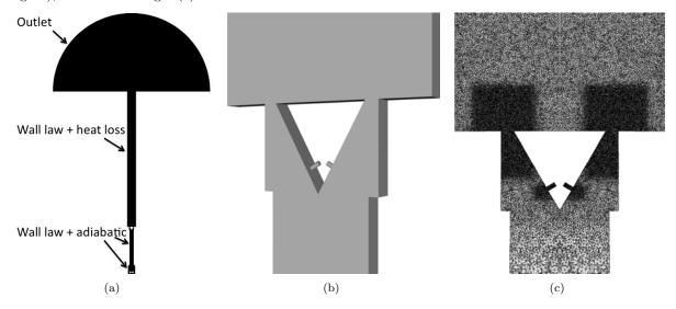
Figure 4. (a) Global view of the computational domain. (b) Close side view of the slice chosen as computational domain. (c) Detail of the mesh around the fuel injection and flame stabilization zones.
