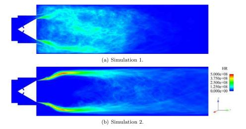
Figure 11. Comparison of mean heat release rate fields between simulations 1 and 2 showing the difference in flame length.
