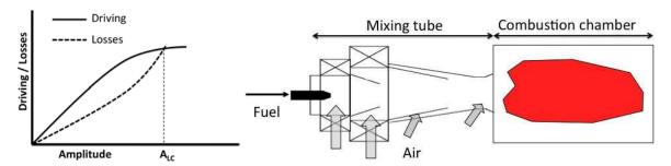
Figure 1. Left: schematic driving and damping amplitudes dependence on the instability amplitude and the resulting limit cycle amplitude  $A_{LC}$ , from Lieuwen [2]. Right: partially premixed flames in LPP systems. In the mixing tube, no combustion takes place. In the chamber, combustion begins in a partially premixed regime.
