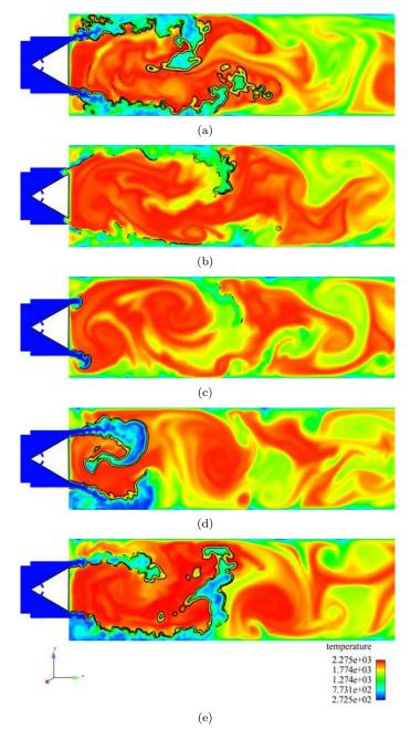
Figure 6. Instantaneous temperature fields and reaction rate isocontours of simulation 1.
