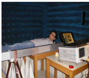
Fig. 15. Image illustrating man 1's measurement in anechoic chamber.
