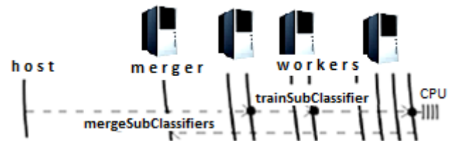
Figure 5. Parallelization of a random forest training. Each subClassifier/small forest is trained over the detected CPU cores through the Weka library
