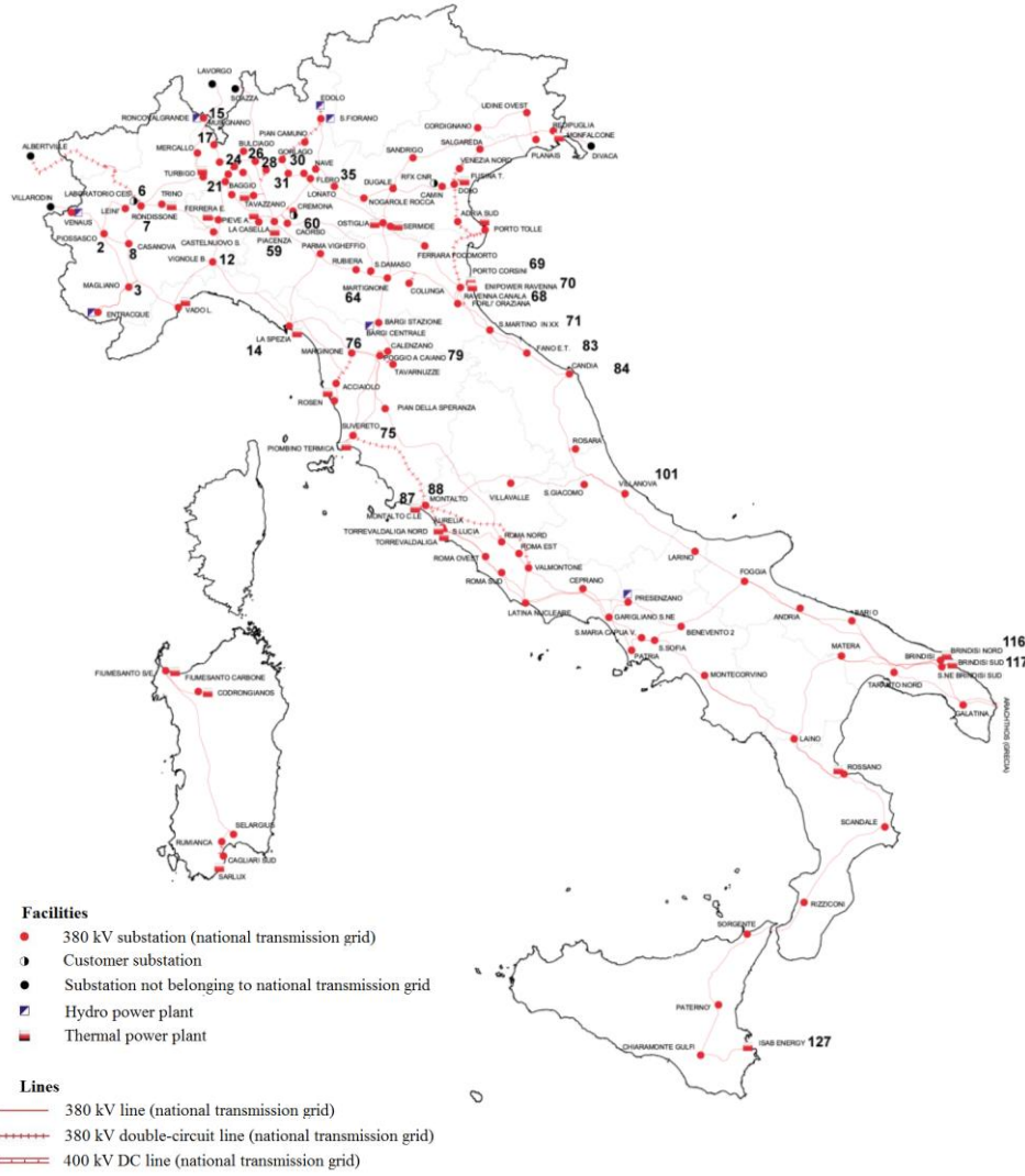
Fig. 1. The 380 kV Italian power transmission network [29], [30].
