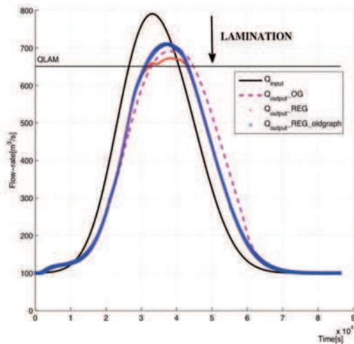
Fig. 10. Comparison of simulation results for  $Q_{lam} = 650m^3/s$ .
