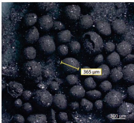
Figure 4 Wear particles of SiC/C tribo-tests.
