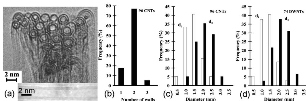
**Fig. 2** (a) HRTEM images of DWNTs and (b) distribution of the numbers of walls for the whole population (established from 96 individual CNTs). Distribution of inner ( $d_i$ ) and outer ( $d_o$ ) diameter for the whole population of CNTs (c) and for DWNTs only (d).
