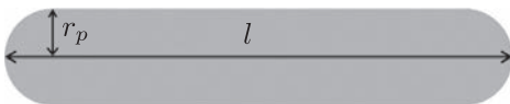
Fig. 4. Needle-shaped precipitates are assumed to comprise a cylinder of length l - 2r_p and radius r_p , ended by two hemispheres of radius r_p .
