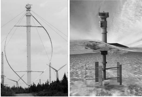
Figure 8.2. Darrieus wind turbine (left) and New Energy tidal turbine (right), with transverse flow and vertical axes
