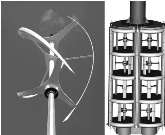
Figure 8.3. Turby wind turbine (left) and Harvest-Ethic tidal turbine (right) with transverse flow
