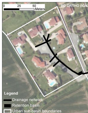
Figure 3: The aerial photography (BD ORTHO® IGN) shows urban cadastral units connected via pipes to the closest sewer system, which leads to the sub-basin delineation (white). The sub-basin is connected to a retention basin. This object-oriented sub-basin delineation does not consider the fact that part of the runoff might not be intercepted in the pipe system but drain to rural sub-basins.
