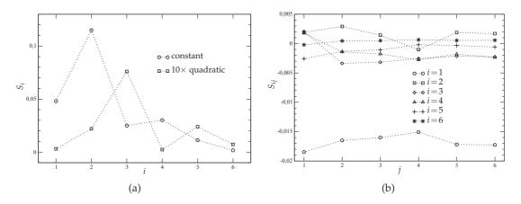
Figure 15: Sensitivity of the actuated coefficients. Constant:  $S_i = \frac{\partial \mathcal{J}}{\partial h_{1i}}$ ; quadratic:  $S_i = \frac{\partial \mathcal{J}}{\partial h_{3i}}$  (rescaled by 10); linear:  $S_{ij} = \frac{\partial \mathcal{J}}{\partial h_{2i}}$ .
