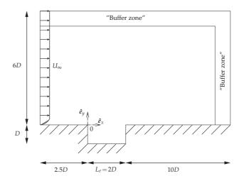
Figure 2: Cavity configuration and computational domain.
