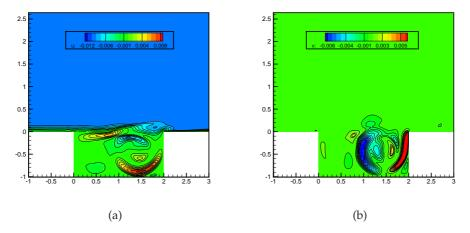
Figure 10: u and v of the difference in the average value  $\delta \overline{q}^{ac}$  between the actuated and the unactuated case.
