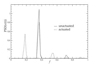
Figure 21: Comparison of Power Spectral Density (PSD) of the original solution and the optimal solution of the normal component of velocity sampled at y=0 and x=1.8D: Actuated (dashed line); Unactuated (continuous line).
