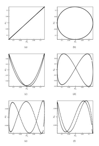
Figure 8: Phase portrait comparison of the first 6 modes, with the POD coefficients:ROM calibrated (solid line), reference POD dynamics (o). POD ROM is calibrated using the  $\mathcal{I}^{(3)}$  minimization for all coefficients. The Tikhonov regularization is applied for (L=0,  $\mathbf{y}_0=0$ ), and the weight matrix  $\Lambda$  based on the overall sensitivity.
