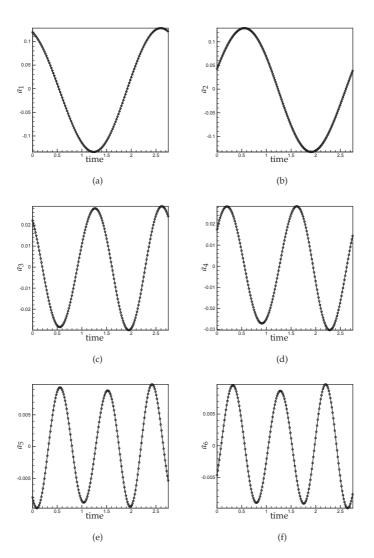
Figure 7: Temporal comparison of the first 6 modes, with the POD coefficients:ROM calibrated (solid line), reference POD dynamics (o). POD ROM is calibrated using the  $\mathcal{I}^{(3)}$  minimization for all coefficients. The Tikhonov regularization is applied for (L=0,  $y_0=0$ ), and the weight matrix  $\Lambda$  based on the overall sensitivity.
