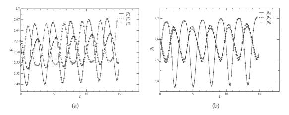
Figure 14: LSE reconstruction of the pressure signals. The pressure value from the sensor are denoted by line, and the coefficients obtained from LSE denoted by  $\circ$  (one over 3  $\circ$  are plotted). The sensors are located at positions (0,D/4), (0,3D/4), (L,D/4), (L,3D/4), (D/2,0), (3D/4,0) along the cavity walls and in the shear layer. Unactuated case.
