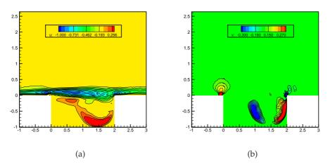
Figure 9: u and v velocity components of the actuation mode  $\psi$  corresponding to an actuation defined by  $v_{wall} = 0.2 \sin(0.4t)$ .
