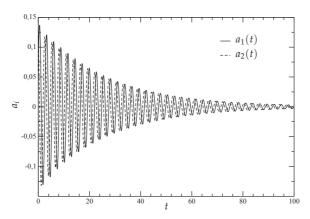
Figure 22: System response of the full system for the state components  $a_1$  and  $a_2$ .
