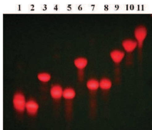
Fig. 3 Denaturing PAGE analysis of ruthenium–DNA conjugates on a Safe Imager™ 2.0 Blue-light transilluminator. Lane 1: 1m ; lane 2: 2m ; lane 3: 2b ; lane 4: 3m ; lane 5: 4m ; lane 6: 4b ; lane 7: 5m ; lane 8: 6m ; lane 9: 6b ; lane 10: 7b ; lane 11: 8b .
