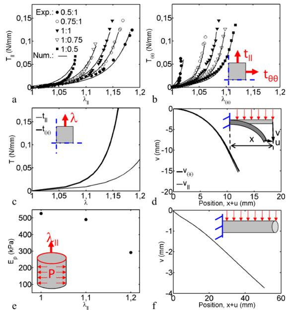
Figure 1: Numerical results for the Gr.2 AAs (a,b): Biaxial tensile tests vs Vande Geest's data (marks) (c) uniaxial tensile tests (d) tissue sample bending test (e) Peterson modulus (f) tube bending test: displacement versus axial position.
