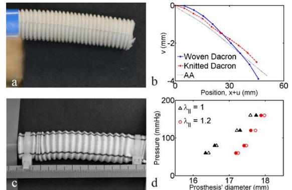
Figure 2: (a) Bending test on prosthesis  $P_1$  (b) Experimental and numerical results: displacement vs position. (c) Inflation test on  $P_2$  (d) Experimental pressure-diameter variations.
