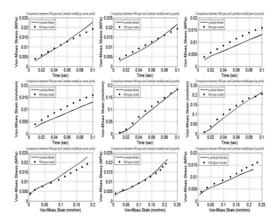
Figure 11. Comparison between a Hill-type model and the  $\lambda$  model for low levels of activation: equivalent stress-strain curves for three selected points on the lips: lip corner, middle point lower lip, and middle point of the upper lip (low activation).
