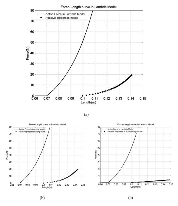
Figure 5. Force-length relations in the DLM: Influence of the passive tissues. For matter of comparison, the solid line curve shows an example of invariant characteristics in the original  $\lambda$  model: (a) Total passive force-length relation along the fibers (dotted curve). (b) Passive force-length relation due to fibers properties. (c) Passive force-length relation due to the properties of surrounding tissues, which corresponds to a simplified Mooney-Rivlin hyperelastic constitutive law.
