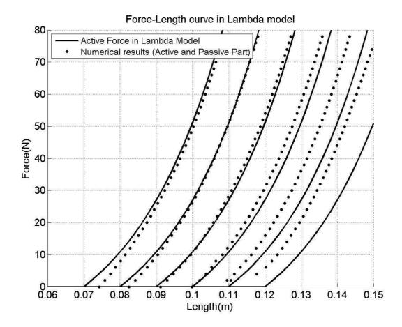
Figure 7. Global force-length curves in the DLM for various  $\lambda$  values (dotted) as compared to the corresponding ICs in the original  $\lambda$  model. The effect of passive properties tends to increase when  $\lambda$  increases, especially when  $\lambda$  becomes larger than the length at rest (0.1 m).
