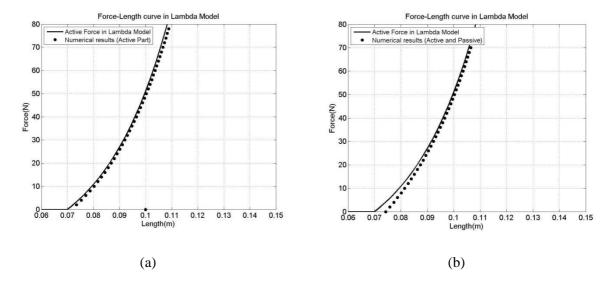
Figure 6. Force-length relations in the DLM - Global assessment: (a) For same  $\lambda$  value, comparison of an example of force-length curve in the DLM (dotted curve) in the absence of passive influences, and of the force-length curve of the original  $\lambda$  model (described in Equation 5) (solid curve). (b) Global force-length curve (dotted lines) including the influence of passive components compared to the force-length curve of the original  $\lambda$  model (solid curve).
