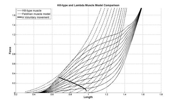
Figure 3 Comparison between the  $\lambda$  model and a Hill-type model: the bold solid path shows an example of force and length variations associated with a voluntary concentric contraction of the muscle (muscle length decreases) caused by changes in motor commands.
