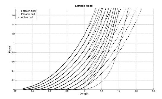
Figure 2. Invariant characteristics (ICs) as defined in the  $\lambda$  model (Feldman, 1986) at constant velocity: the dashed curves depict the passive force-length relations; the solid curves depict the global force-length relations after addition of the active parts (dotted curves) to the passive characteristics.
