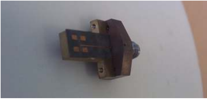
Figure 15. The antenna array mounted on a cylindrical skin-equivalent phantom (the total antenna size without connector was 8 mm × 20 mm).
