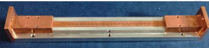
Figure 27. The prototype of the substrate-integrated waveguide-slot antenna.
