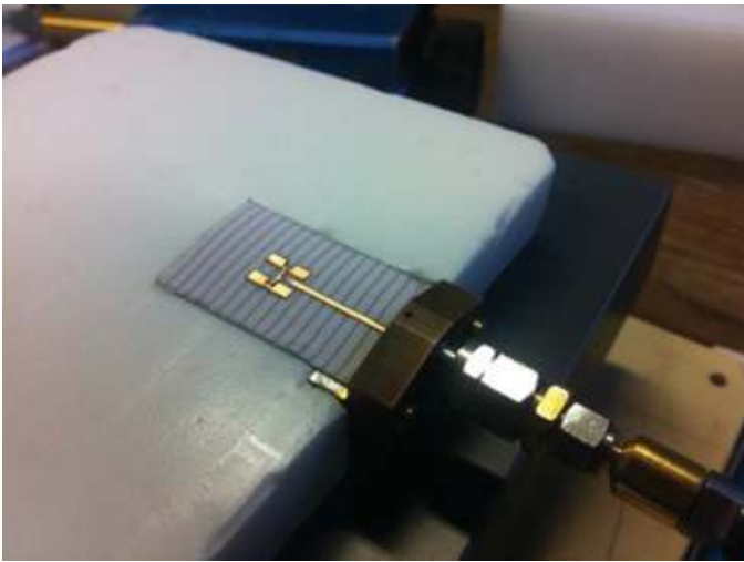
Figure 17. The textile antenna array mounted on a paralleliped skin-equivalent phantom.
