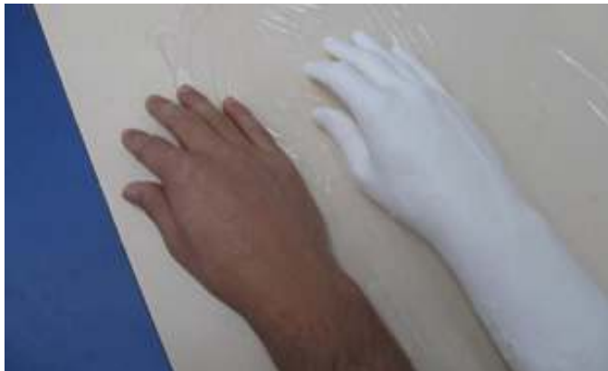
Figure 7. A skin-equivalent phantom representing an arm and a hand: (left) a human arm used to make a realistic mold; (right) the phantom.
