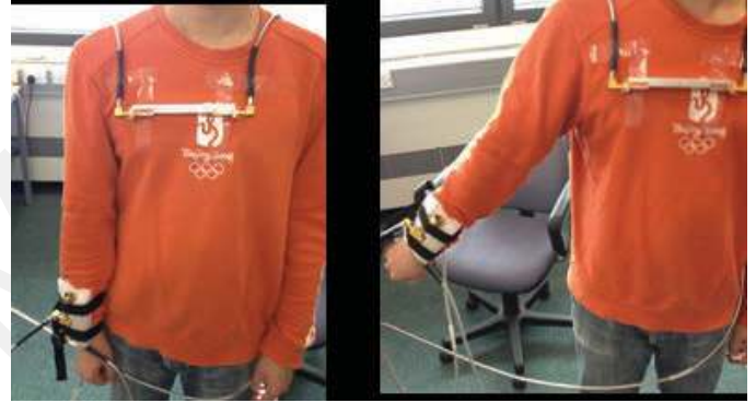
Figure 32. The antenna placements for the wrist-chest channel measurement and body posture (40°).
