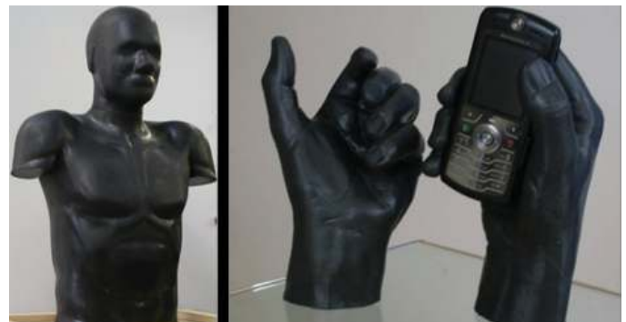
Figure 8. Solid phantoms made of carbon-loaded silicon rubber (reproduced from [60]).
