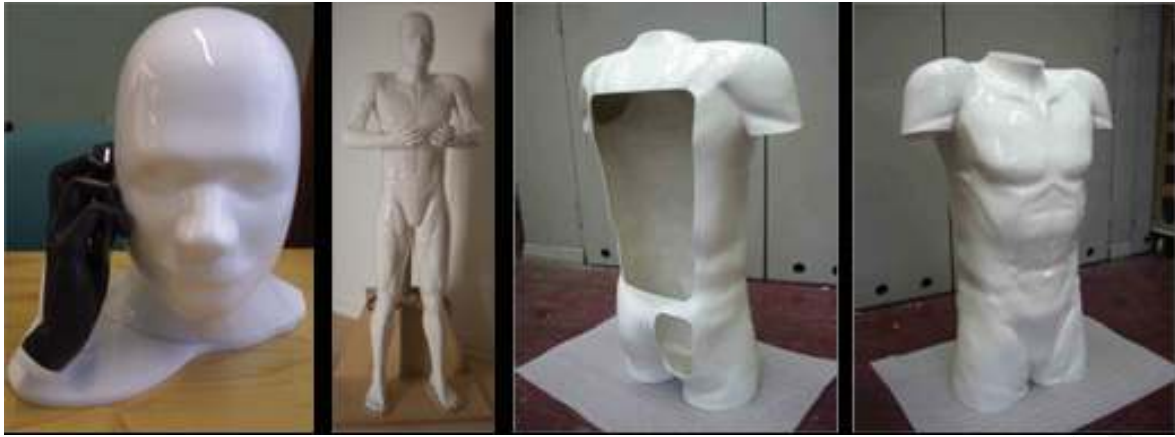
Figure 6. Shells for liquid phantoms (reproduced from [60]).
