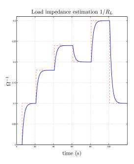
Figure 6: Simulation result of the load admittance estimation.
