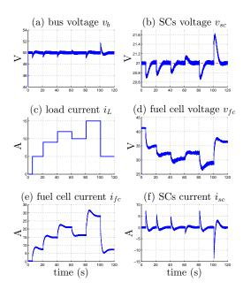
Figure 12: Experimental result during a step load with an integral action ( $\alpha$ =10,  $\gamma$ =460).
