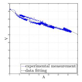
Figure 3: Fuel cell voltage vs current.
