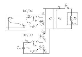
Figure 4: DC bus and load model.
