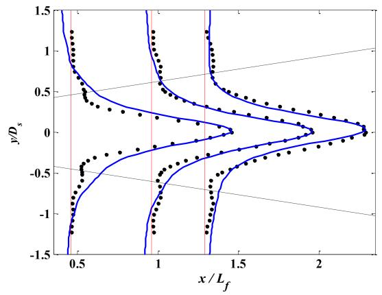
Figure 3: Experimental profiles of normalized acoustic intensity (dots) and normalized axial velocity (solid blue lines) along the y axis at  $x = 0.5L_f$ ,  $x = L_f$  and at  $x = 1.3L_f$  for an acoustical power of 2.8W. The two dash-dotted lines correspond to the diffraction cone (equation (14)). Note that the scale is very different on the y-axis and on the x-axis, so that this figure represents in fact a very elongated region, since  $L_f = D_s^2/\lambda >> D_s$  in our experiment.
