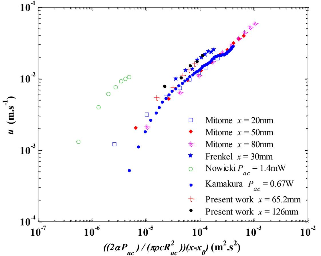
Figure 4: Test plot of equation (19). Velocities measured in several former studies plotted as a function of the group appearing in the square root on the right hand-side of equation (19).
