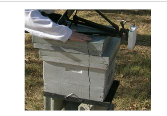
**Figure 2: Stereo vision camera.** A stereo vision camera capturing the entry of a beehive including the entire flight board.
